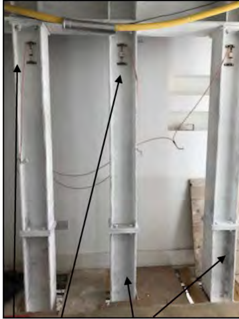
Strain sensors: attached to props (steel support columns)
