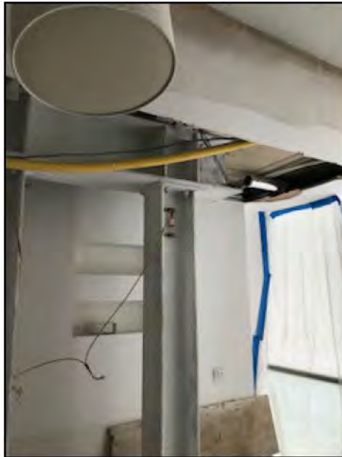
Strain sensors: attached to props (steel support columns)
